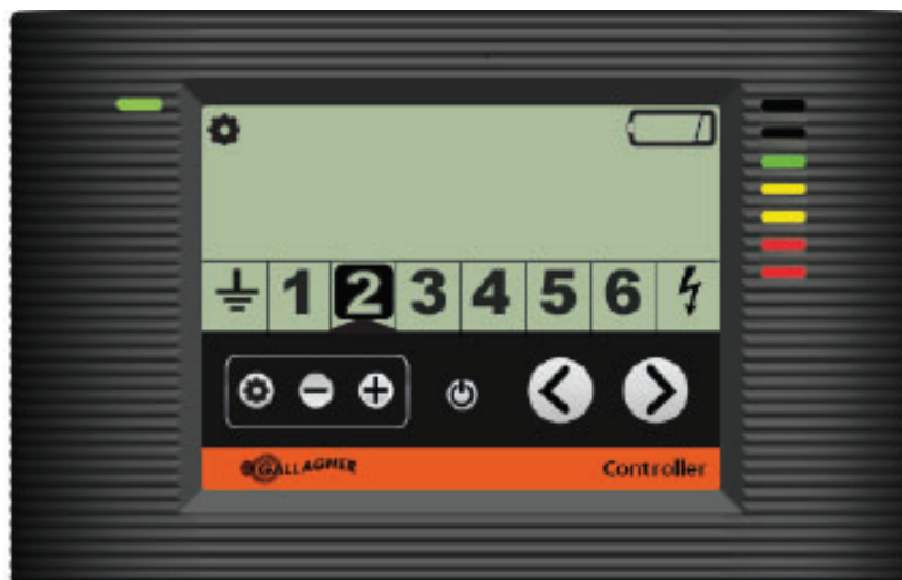
Controller showing zone 2 with a low battery
