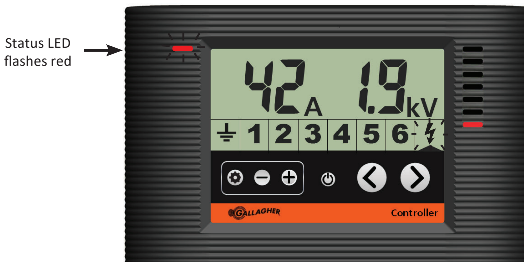
Controller showing the energizer in current alarm
